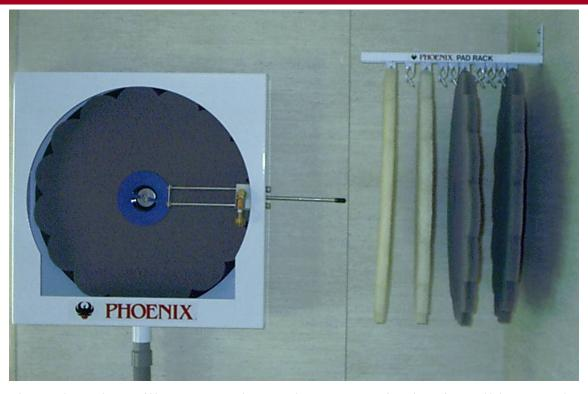
The pad washer will accommodate pads up to 24" in size, is wall hung and comes with a mounting bracket. The force of the water spins the pad, which helps to dry it. The unit should be installed near a drain and hot water supply. When used with Phoenix Blast Pad cleaning chemical, you have a very effective and quick way to clean dirty pads. Also shown in the picture is the Phoenix Pad Drying Rack.
